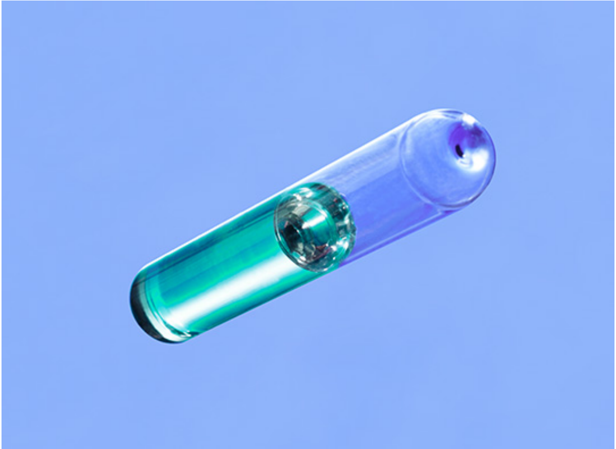
Very thin-walled ampoule for larger volumes
